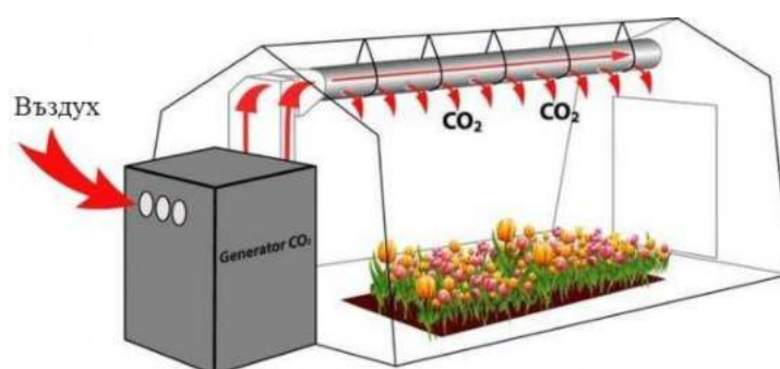
Figure 5. Schematic diagram for supplying CO 2
